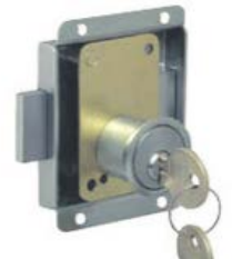
latch #3273Z; 25 mm backset, brass chrome plated; also with 20, 30 mm backset For door thickness from 5/8" to 1 3/16."
